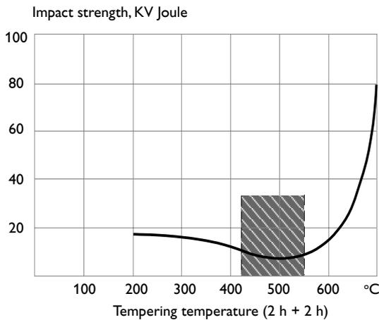
Tempering within the range 425 – 550 °C is normally not recommended due to the reduction in toughness properties avoided.
