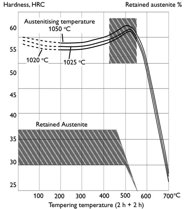
Above tempering curves are obtained after heat treatment of samples with a size of 15 x 15 x 40 mm, cooling in forced air. Lower hardness can be expected after heat treatment of tools and dies due to factors like actual tool size and heat treatment parameters.
