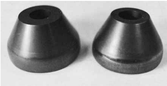
PVD coated tools in ASSAB PM 23 SuperClean for cold forming of tubes.
